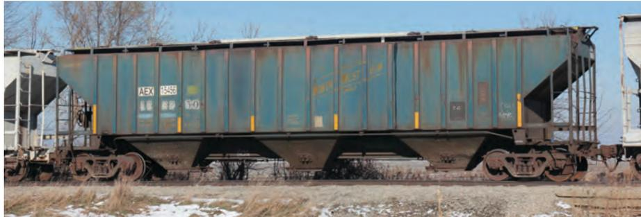
Reflective strips applied to AEX covered hopper. Reflectors have been applied in vertical manner closely matching FRA guidelines. Reference images of the prototype are very helpful in determining exact reflector placement.
